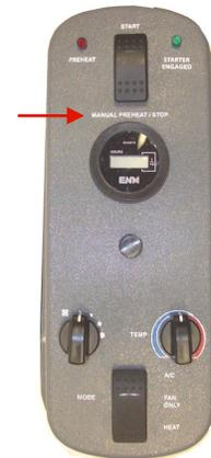
**The Glow Plug Operates When the RED light comes on. Hold down the button until the green light shines and the engine starts.**
