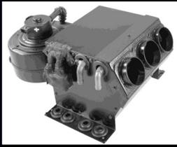
Under bunk unit with A/C and Heating coils inside.
